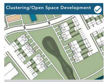
Concentrating buildings and impervious surfaces on a portion of a site allows other areas to remain natural. This reduces stormwater pollution, construction costs and the need for regrading.
